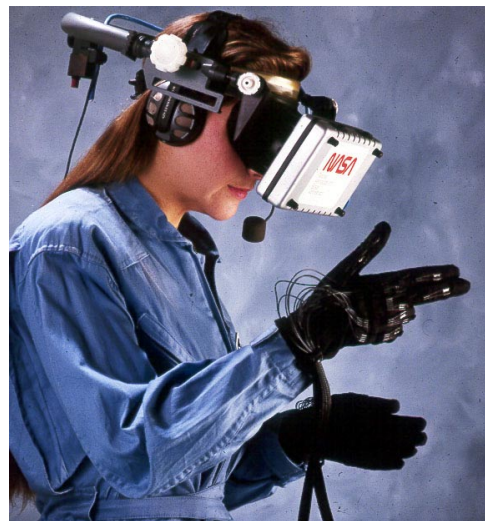
Figure 1. Virtual Interface Environment Workstation Project (VIEWlab) at NASA Ames Research Center, 1988. VIEWlab System including helmet nounted display with 3D sound, speech recognition, and dataglove. (Photo credit: NASA/W.Sisler, S. Fisher, 1988)
