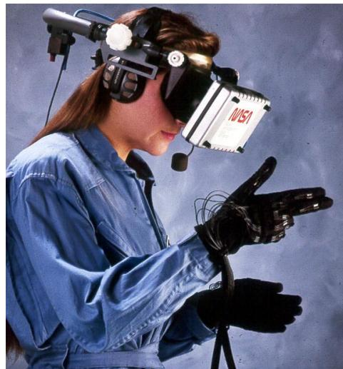
**Figure 1. Virtual Interface Environment Workstation Project (VIEWlab) at NASA Ames Research Center, 1988. VIEWlab System including helmet mounted display with 3D sound, speech recognition, and dataglove. (Photo credit: NASA/W.Sisler, S. Fisher, 1988)**
